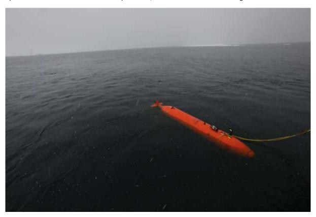
Photo 2, Caption: The University of Gothenburg's Kongsberg HUGIN AUV 'Ran', shown here, being launched in an open water polynya at Thwaites Glacier. The sub would be programmed to undertake 20-hour missions, combining programs of sea-floor mapping and mid-water column profiling and sampling, at and under Thwaites Glacier ice shelf.
