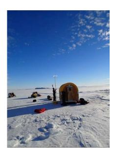
Photo shows an equipment station on McMurdo Sound fast ice. The Conestoga Wagon on a sled contains computers and navigational equipment for the underwater SCINI ROV and acoustic and fluorescence sensors that were deployed thorough holes drilled in the sea ice.
