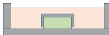
Figure 4. Sample setup. The inner crucible (gray) holds the sample pellet (green), which is surrounded in the outer crucible by the redox buffer (pink).
